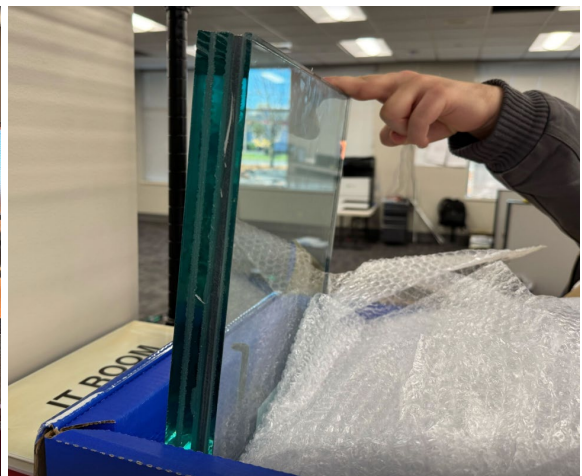
Left: Arrows showing 8ft high Level 4 Ballistic Panels in place Right: Sample Level 4 Ballistic Glass Window. The ballistics are so heavy they needed to construct reinforcements to hold the weight. We will keep non-ballistic windows on the exterior so everything matches.
